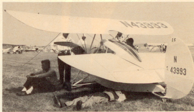
A modified Flying Flea, Model ME-2Y, built by Frank Easton of Salem, O., in 1945. Powered by a 40 h.p. Continental A40 engine and fitted with a cockpit canopy, this one features an elevator built into the trailing edge of the rear wing. Now in EAA Museum, Hales Corners, Wis.
