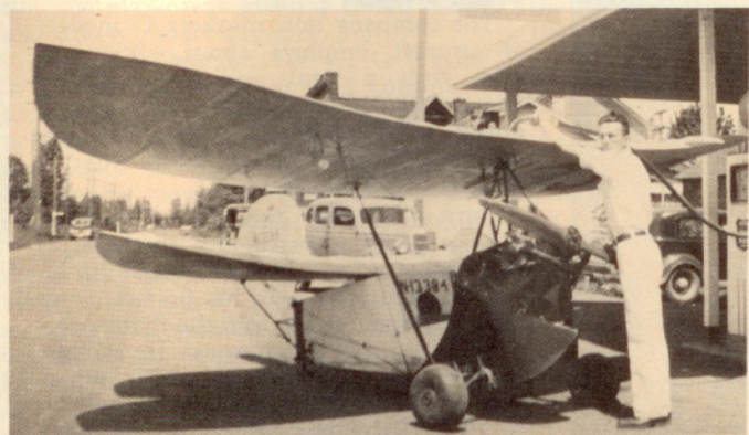
An American-built Flea powered by a 32 h.p. British Bristol Cherub airplane engine. Pilot Myron Buswell taxied this one right up to his brother's gas station in Tulatin, Ore., circa 1939.
